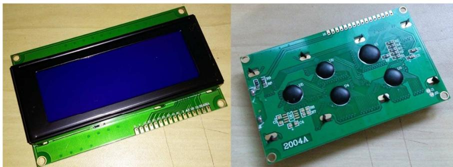
Figura 6 LCD 2004 20x4 Display
